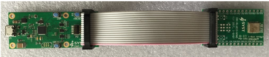
Figure 7: IDAP-Link JTag with IBK-BLUEIO-NANO for development with the IMM-NRF52832-NANO module
